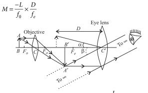
Magnification due to objective,  $m_0 = \frac{L}{-f_0}$
